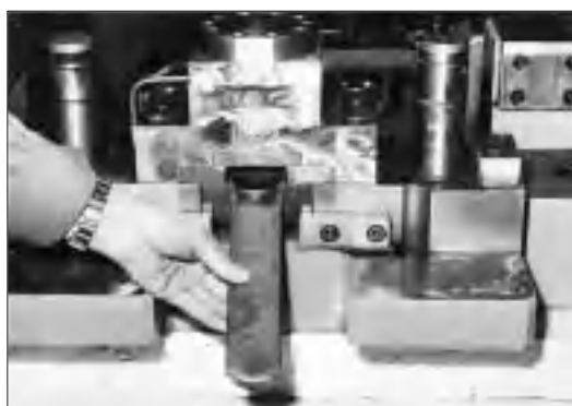
Cold cropping tool made from Uddeholm Viking.
