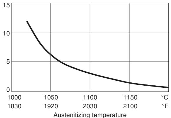
*\*) Holding time = time at austenitizing temperature after the tool is fully heated through.*
