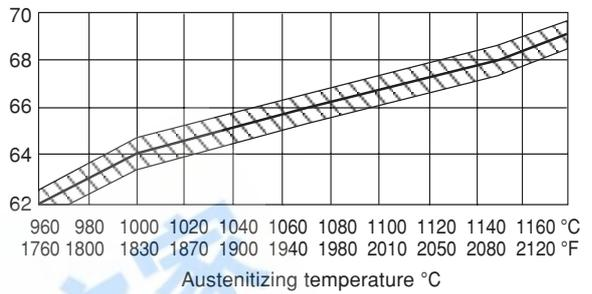
*Hardness for different austenitizing temperatures after tempering 3 times for one hour at 560° C (±1 HRC).*
