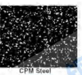
The CPM process results in a finer, more uniform carbide distribution imparting improved toughness and grindability to high alloy steels. The CPM process also allows the design of more highly alloyed grades which cannot be produced by conventional steelmaking.
