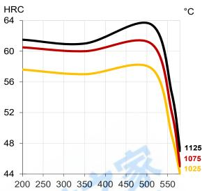
Tempering temperature in °C Hardness after hardening, quenching, cryogenic treatment and tempering
