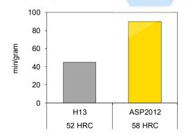
Wear resistance is measured as the time needed for removal of one-gram material from a test piece.
